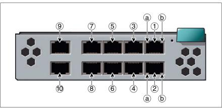
Figure 39: Control and connection panel of the Ethernet LAN Pass-Thru-Blade
